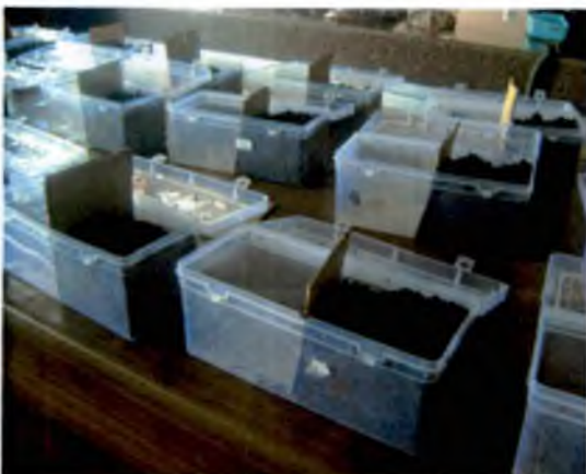
3. Soil were placed on the two sides of containers
