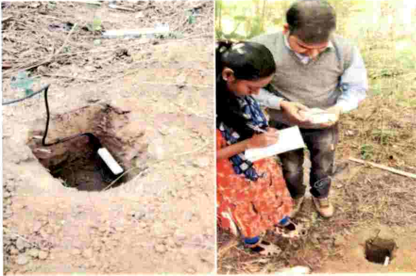
Plate 17: Taking reading from installed probe at 15cm
