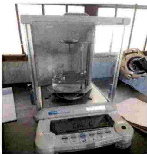
Precision electronic balance (Shimadzu AUY 220)
