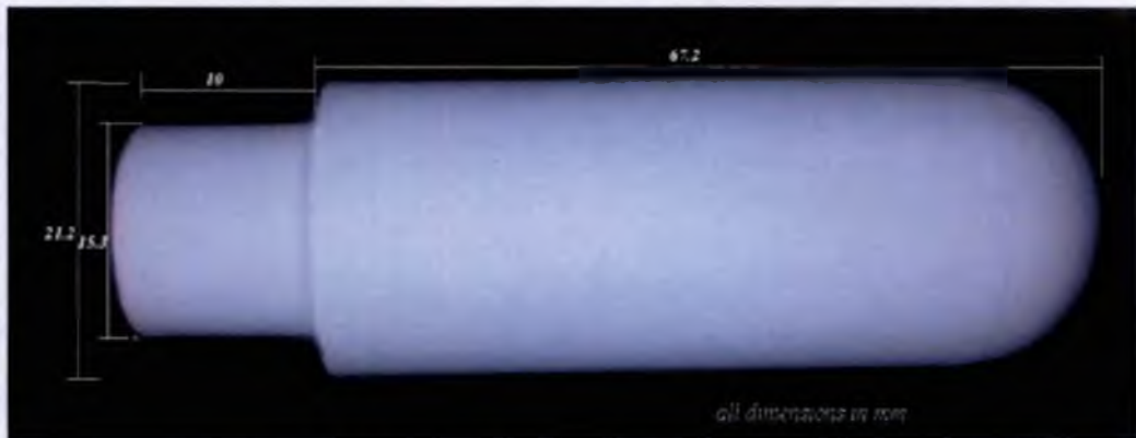
Plate 4.5 Tensiometer porous cup used as sensor
