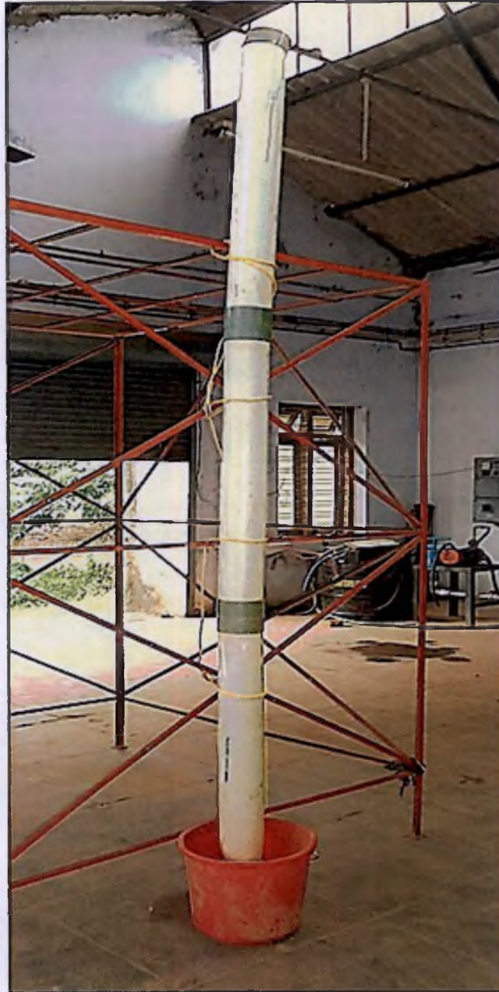
Plate 3.1 Experimental setup for determining the Wetting Curve
