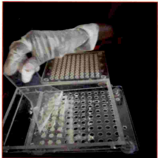
Step 6. Spreading filler material
