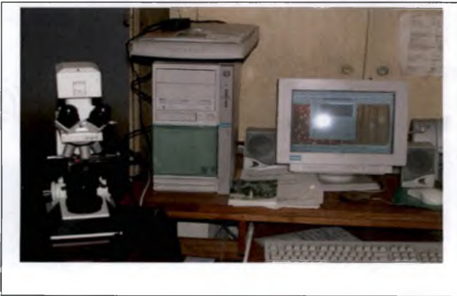
Plate 25. Image Analyser (Labomed Digi-2) used for anatomical quantification
