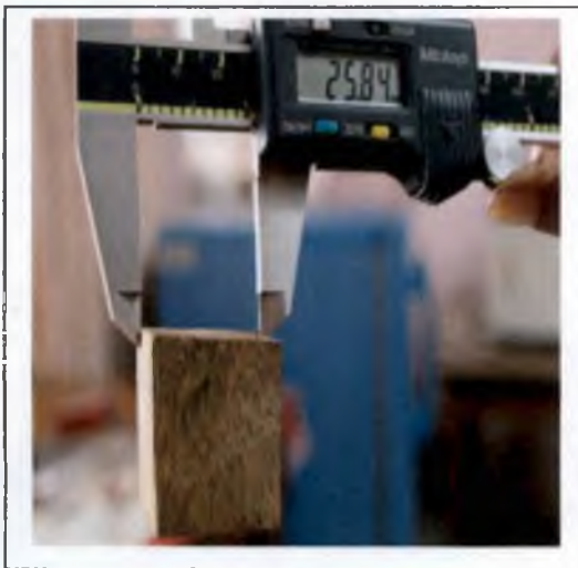
Plate 18. Measurement of radial length for assessing shrinkage using vernier calliper
