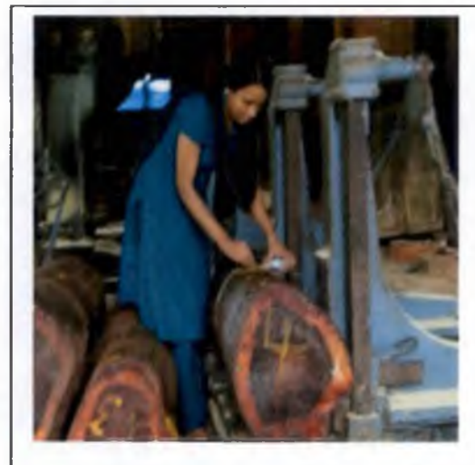
Plate 19. Measurement of mid girth of Andaman padauk logs for assessing log volume
