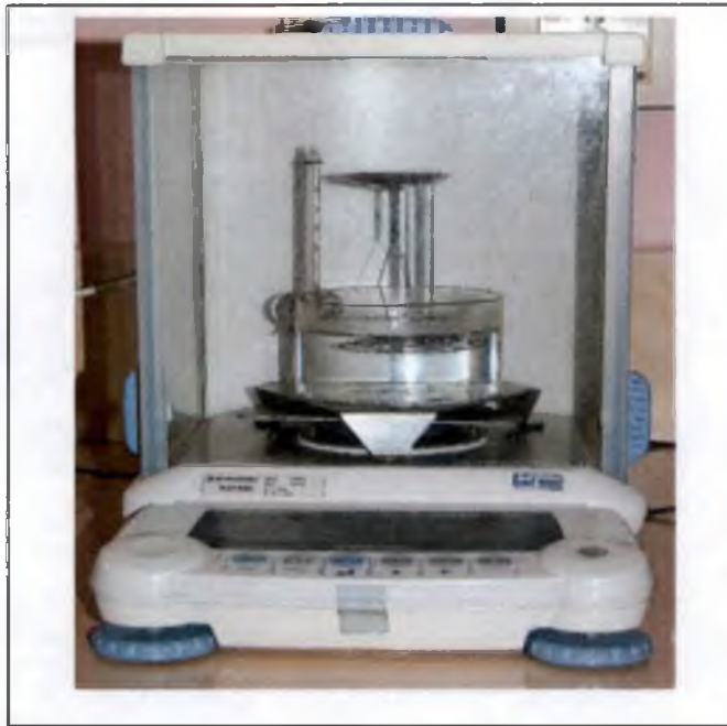
Plate 24. Specific gravity module attached to an electronic balance
