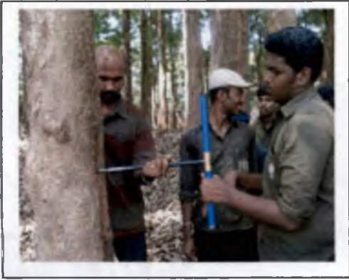
Plate 20. Collection of increment core samples using Haglf increment borer (CO1512) for studying anatomical parameters
