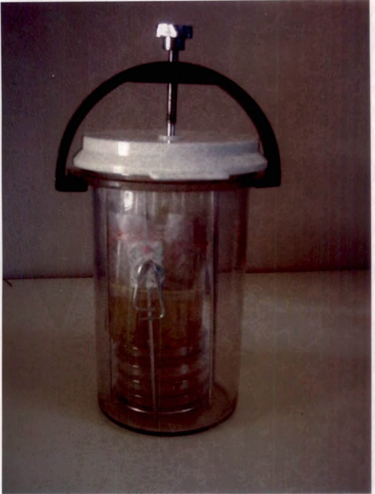
Plate 1. Rolling tubes and pour plates incubated inside anaerobic jar
