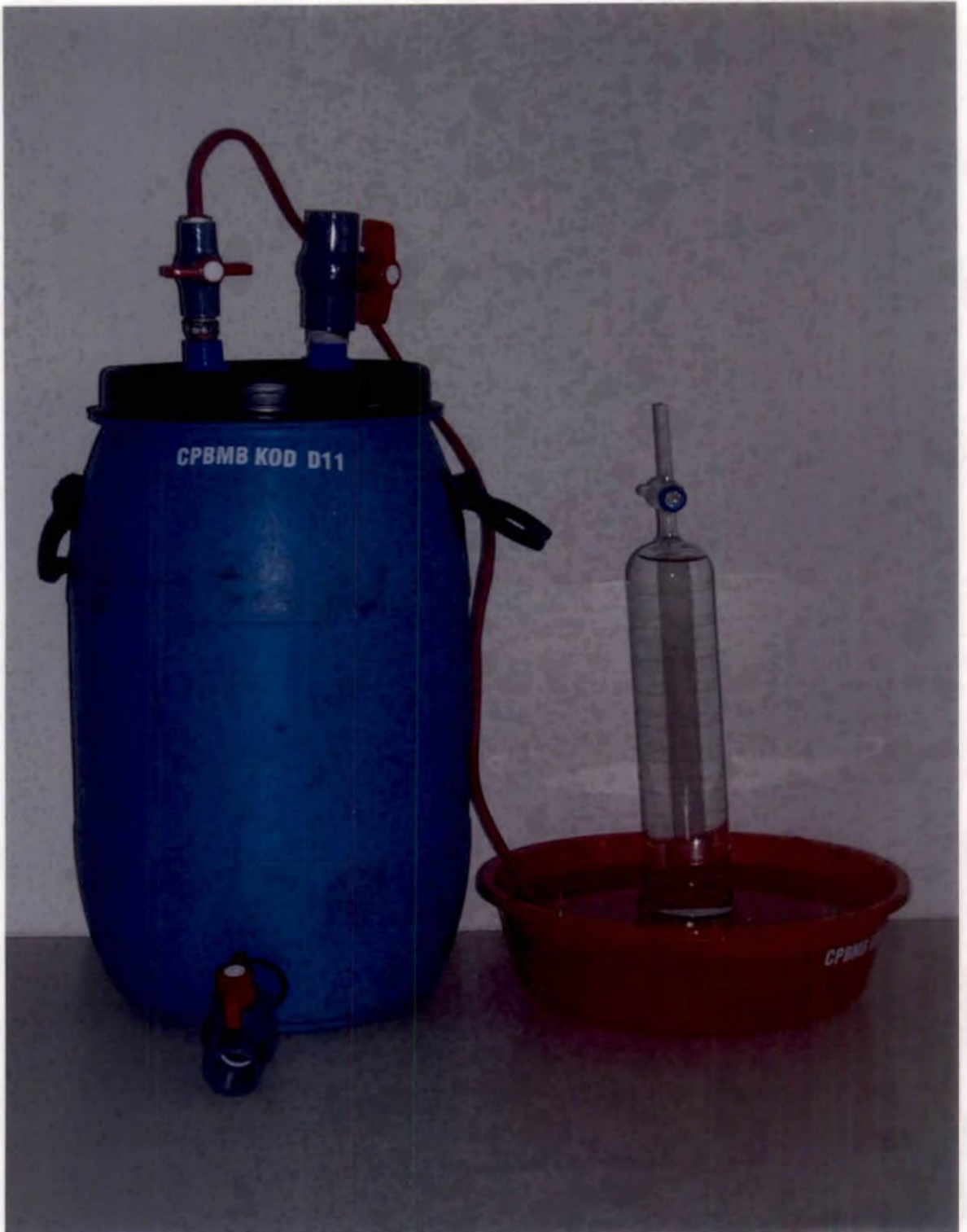
Plate 2. Experimental biogas unit
