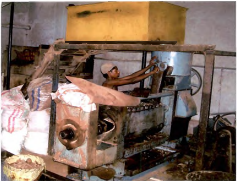
Plate 8. Coconut oil extraction by coconut oil expeller
