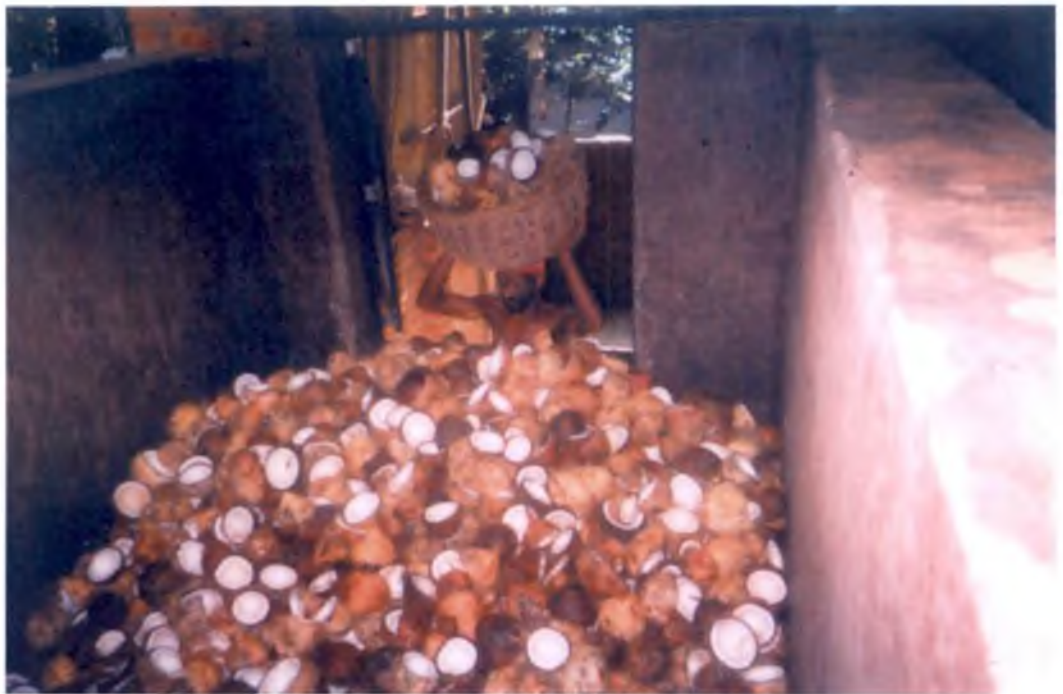
Plate 2. Splitted nuts fed into drying chamber of copra drier
