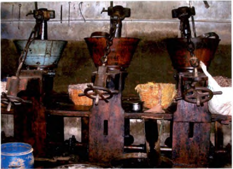
Plate 7. Coconut oil extraction by mechanical rotary chekku
