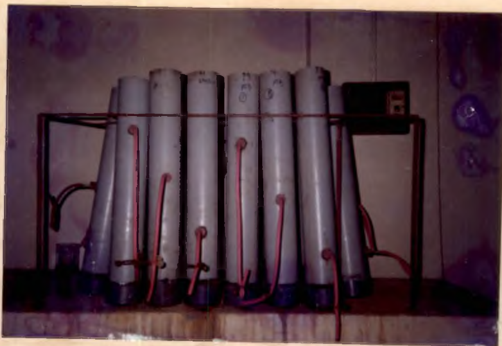
Plate 3. Arrangement of columns for leaching study
