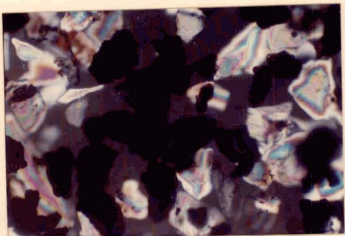
38. Primary mineral assemblage of soil gravel fraction - (2.5-7.5cm)-(62-150cm) - light fraction - Nedumangad series - under crossed nicols - Mgf: x 63.
