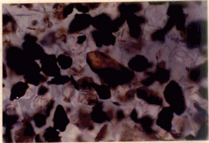
137. Fine sand mineralogy of soil - (0-14cm) - light fraction - Trivandrum series - in plane light - Mgf: x 63.
