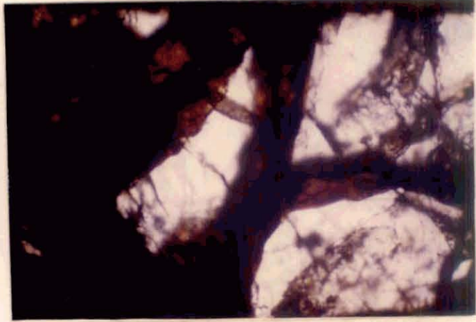
89. Micromorphology of soil gravel - (2.5-7.5cm)- (62-150cm) - Nedumangad series - in plane light - Mgf: x 25.
