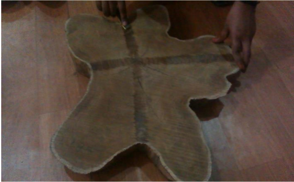
Plate 2. Preparation of discs to obtain surface for measurement
