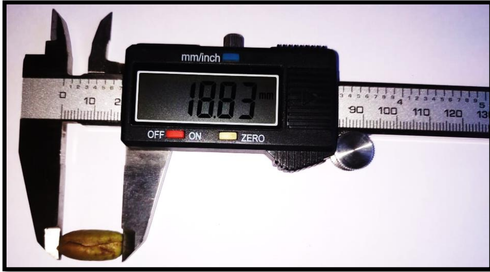
Plate 6. Measuring Seed length by Digital Vernier Caliper (HAWK HT0472)
