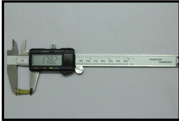
Plate 4. Measuring mature bud length by Digital Vernier Caliper (HAWK HT0472)
