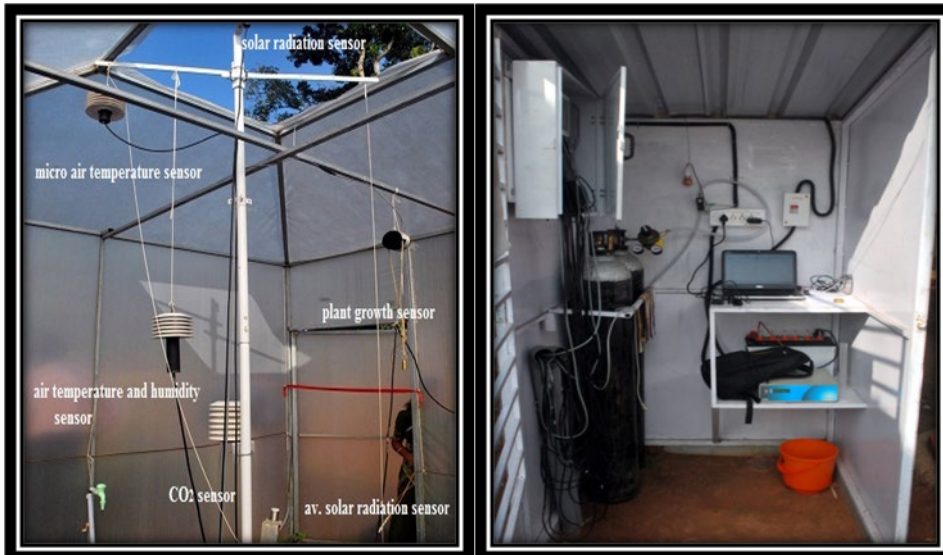
Plate 2. Various sensors and CO 2 cylinders used in Open Top Chamber
