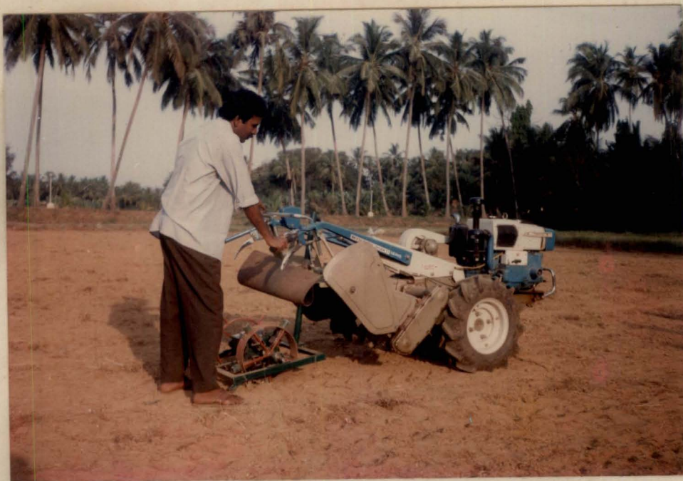
Plate 3.8 Jab type paddy dibbler with power-tiller in operation
